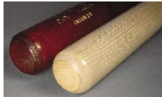
The colorful maple bat, left, and the composite bat (wood wrapped in a fiberglass mesh, then soaked in resin), right, are departures from baseball's traditions. Note the cupping at the end of the composite bat.
