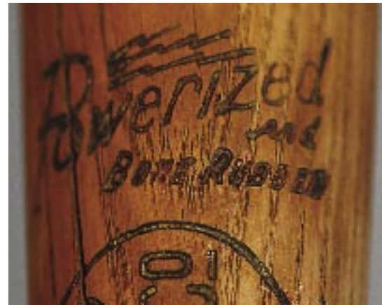
This bat from the mid-1930s shows two Louisville Slugger processes: "Powerized" and bone-rubbed. Rubbing a bone on the bat while it was still on the lathe for even a minute or two would take the place of a player doing this by hand for many hours.
