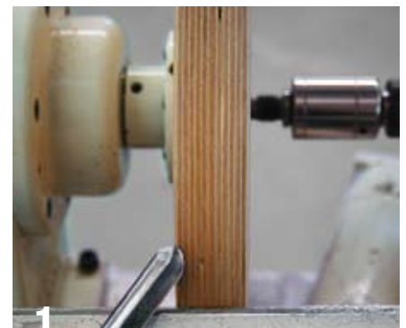
Trim the glued up disc gently from both ends to create a cylinder. Sand it smoothly, being sure there are no sharp corners.
