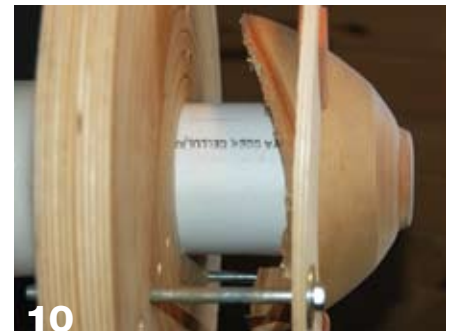
10 By using a short section of thick-walled Schedule 40 PVC, you can turn the bottom of natural-edged bowls with the Straka chuck. With both ends squared, the pipe sets about ½" into the base.
