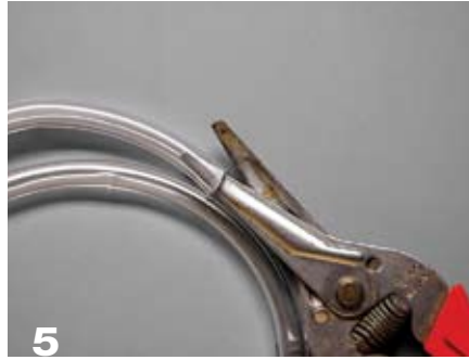
5 To pad a ring with clear plastic hosing, cut through the top of the natural curve of the hose. When cut like this, the natural spring of the hose will hold it inside the opening.
