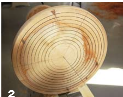
2 Draw lines about every \frac{1}{2} ". Cut into these lines lightly with the long point of a skew or corner of a parting tool. Divide the disc into three equally spaced sectors.
