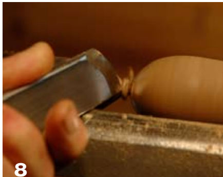
8 With the long point of the skew, make a series of V-cuts to part the handle from the lathe.
