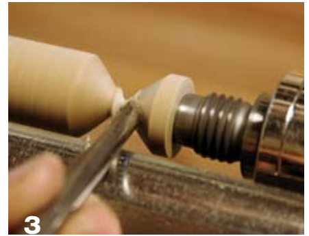
3 One option: Turn a cone that fits on the end of your cup center. The cone should taper down to a diameter less than \frac{3}{8} ".
