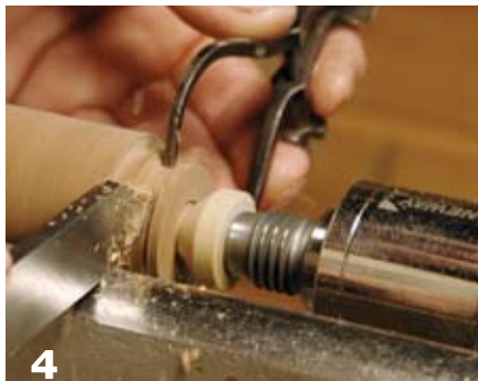
4 With a parting tool and calipers, size the tenon with the lathe running. Set the calipers to the outside diameter of the ferrule.
