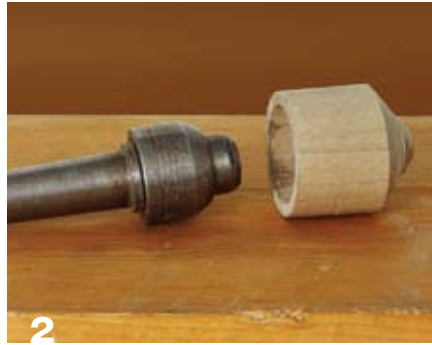
2 If you don't have a cone center, turn shop-made cone-shaped covers to fit over your revolving cups.
