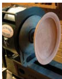
Above: The inside of the Vicmarc VO1343 includes belts, adjustable counterweights, and adjustments for the proportions of the oval. Right: Turning stock attaches to the device with a standard 4-jaw chuck or faceplate.
