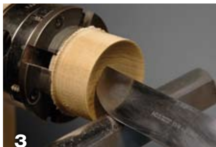
A finishing technique to remove small amounts of wood is often called "shear scraping." The tool is no longer flat on the rest but canted in the direction of the cut at around a 45- to 70-degree angle.
