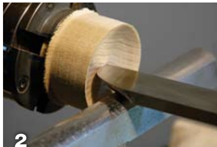
In "normal" scraping, the tool is held flat on the tool rest (positioned close to the work) with the handle raised slightly in back and with only the edge contacting the wood.
