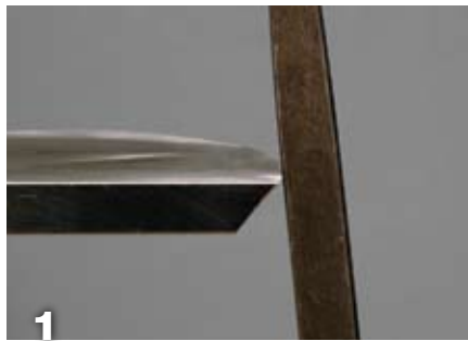
To pull a burr with a burnisher or a diamond hone, steady the tool and present the burnisher (triangular, oval, or round) at a 3- to 5-degree tilt toward the top of the tool. Make one steady pass. The amount of pressure you apply changes the burr from light to heavy.
